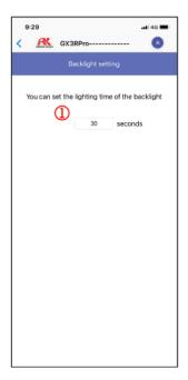
① This is used to set how long the backlight stays lit. Setting range: 0 to 255 seconds
