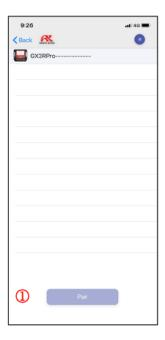
Detects and displays the device names of any detectors in the vicinity of your smartphone. Select a device name and tap the 1 Pair button to pair with that device. The display returns to the top screen if no gas detector is found within a preset time.
