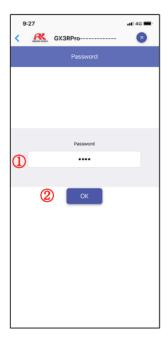
This is used to enter the user password for the detector required to modify the detector settings.
