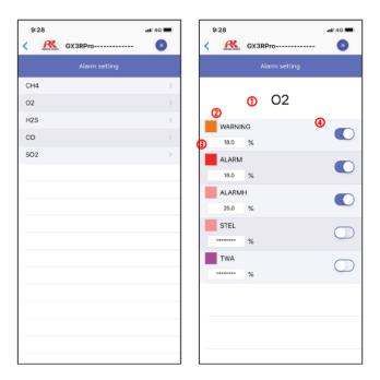
Displays the names of the gases currently being measured. Select the gas name to display the Alarm setting screen for the gas.
